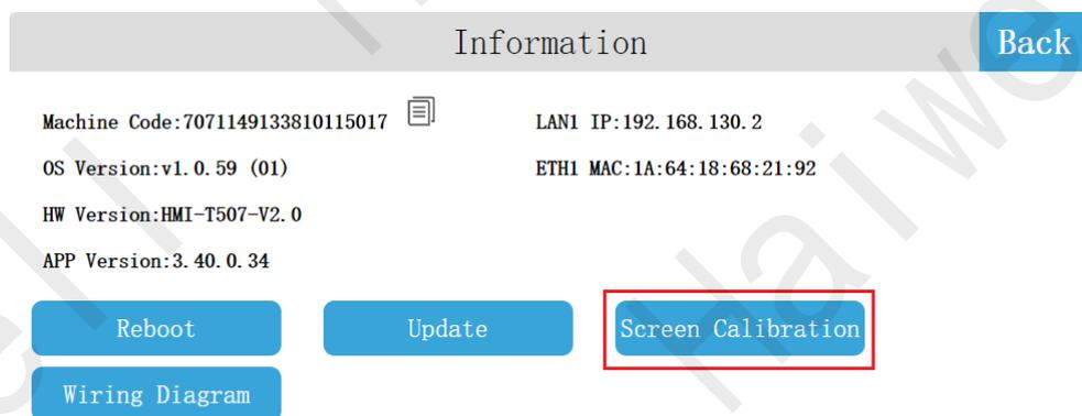
Figure 146 Click to start touch screen calibration
